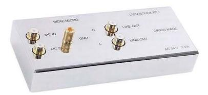
The small size of the PP-1 allows close placement to the turntable, minimizing signal leads from the tonearm. The whole power supply is inboard the PP-1 chassis except for an external power transformer, which is outboard to eliminate magnetic field interaction.
